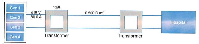
(a) Explain the advantage of using a step-up transformer before transmitting electrical power over any significant distance. (3 marks)
