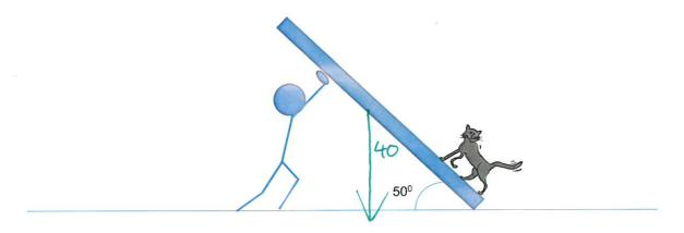
(a) The bookshelf is 2.40 m tall with a uniformly distributed mass. The man is pushing with a maximum force of 270 N at a distance of 0.600 m from the top end of the bookshelf. Calculate how far up from the bottom end of the bookshelf the cat can walk before the man is unable to support it.
