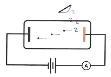
The required stopping voltage (V) to reduce the current reading in the ammeter to zero for a variety of light frequencies was recorded.
